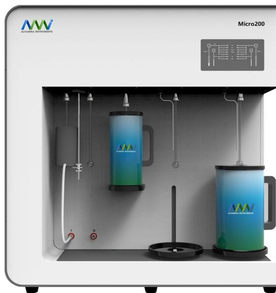
The AMI Micro 200 Series can accurately produce surface area and pore size results of powder materials. These instruments are divided into three types: A, B, and C, and the C type is configured with 1 torr or 0.1 torr high-sensitive pressure sensors and a turbo molecular pump with ultimate pressure of  $10^{-8}$  Pa. The C series can effectively perform an analysis of microporous materials such as: molecular sieve, catalyst, activated carbon, and other microporous materials.
